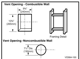
Fig. 17 Locate vent opening.
